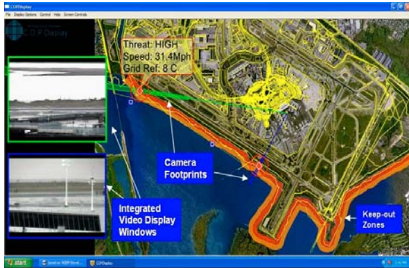
Figure 3: The Common Operational Picture display shows a high resolution map with camera videos that form a single integrated security picture. Camera footprints are color-coded to match the associated video windows and keep-out zones are delineated by level of alert (yellow is warning, red is alarm). Information for a hooked track is shown in the call-out bubble.
